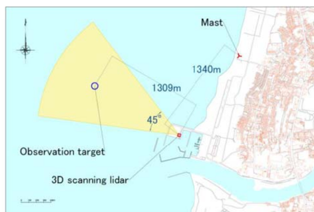
Fig. 1 Location of the 3D lidar and the met mast
