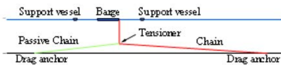
Fig. 5 Overview of holding power test
