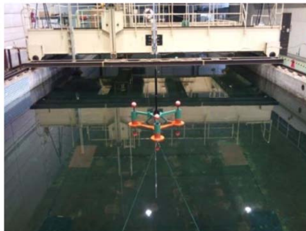
Figure 8. Overview of the water tank and platform.
