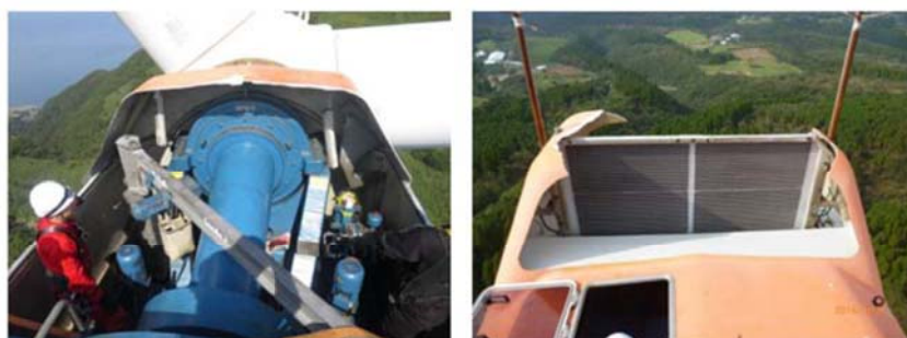
FIGURE 1 Damage to the nacelle cover during the typhoon at Minamiosumi wind farm 12 [Colour figure can be viewed at wileyonlinelibrary.com ]
