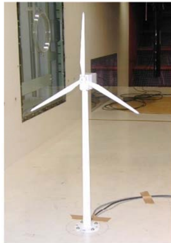
Fig. 1. 1/100 scale model wind turbine in the wind tunnel test and its dimensions.
