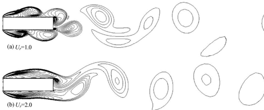
Fig. 13. Instantaneous vorticity field of a B/D=4 cross-section in transverse forced vibration with y_0/D=0.02 at its maximum lift.
