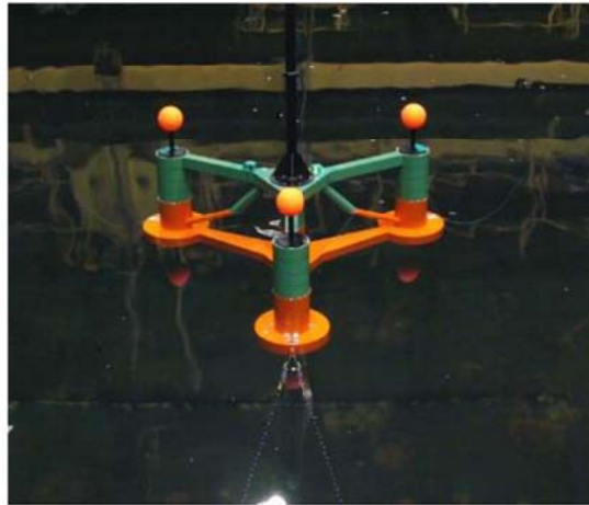
(a) Overview of the semi-submersible model in the water tank test
