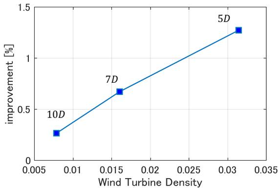
Figure 7. AEP improvements versus wind turbine density
