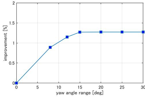
Figure 6. AEP improvements versus the yaw offset limit.
