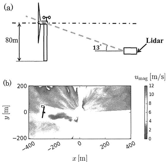
Figure 7. (a) Schematic of a conical scan at an elevation angle of  $13^\circ$ . The lidar beam hit the nacelle at this angle. (b) Velocity magnitude of the conical plane at the elevation angle of  $13^\circ$ .
