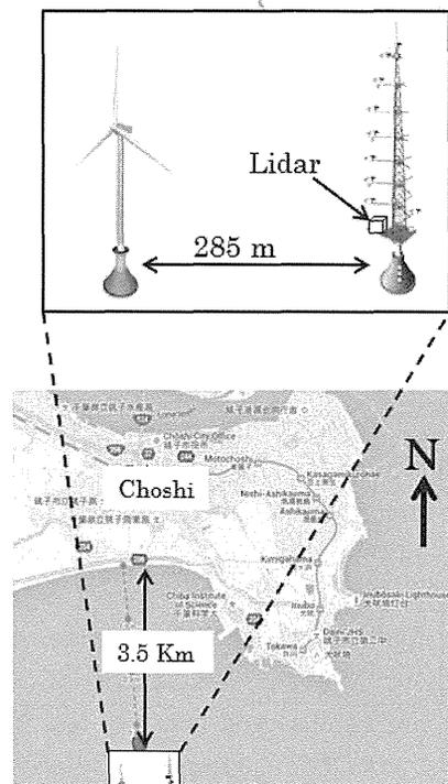
Figure 1. Google map of Choshi offshore site. The zoom in shows the location of wind turbine, observation tower and the scanning lidar.
