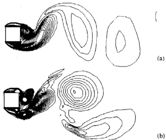
Fig.3 Instantaneous vorticity contour of a rectangular cylinder with B/D=1.0 . (a)CASE1:k-ε model+2layer, (b)CASE2:3rd-order upwind(K-K) only. Re=2.2 \times 10^4
