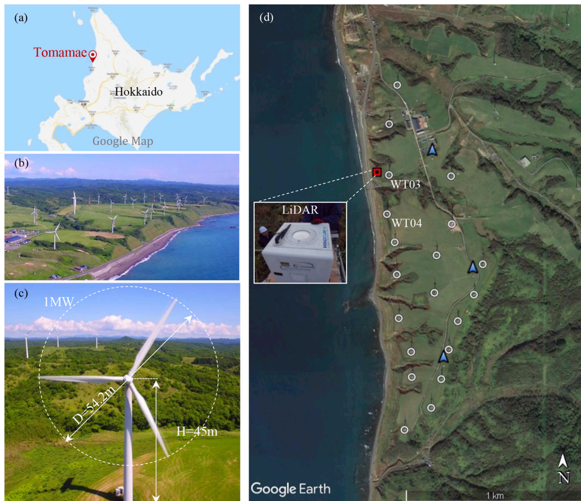
Fig. 2. Test site in the Tomamae wind farm: (a) location of Tomamae; (b) aerial picture of wind farm; (c) wind turbine and its dimensions; (d) layout of the wind farm and measurement where the white open circles denote the location of each wind turbine and the red square indicates the position of LiDAR. (For interpretation of the references to colour in this figure legend, the reader is referred to the Web version of this article.)
