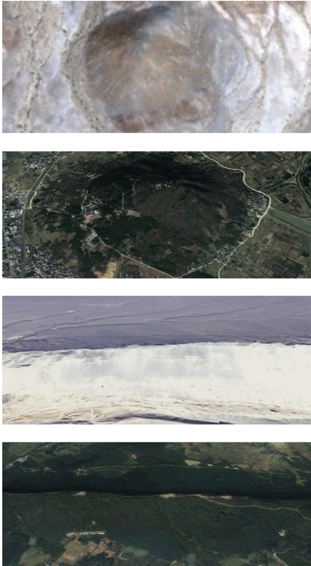
Fig. 1. Typical topographies, (a) smooth 3D hill, (b) rough 3D hill, (c) smooth 2D ridge, and (d) rough 2D ridge.
