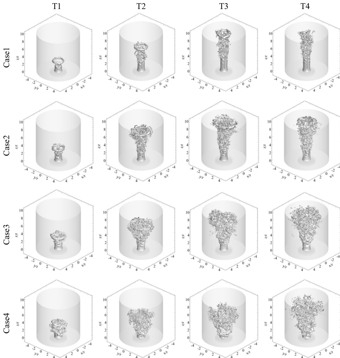
Fig. 5. Iso-surface of the second eigenvalue, \lambda_2 = 0 , of the tensor M = S_{ik}S_{kj} + \Omega_{ik}\Omega_{kj} , for Case1, Case2, Case3, and Case4 at time of T1, T2, T3, and T4. Cartesian coordinates have been normalized by the radius of the chamber outlet r .
