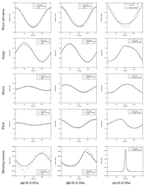
Figure 6. Comparison of time histories of normalized elevations, dynamic responses and mooring tensions, by linear and nonlinear wave theories for different wave heights.
