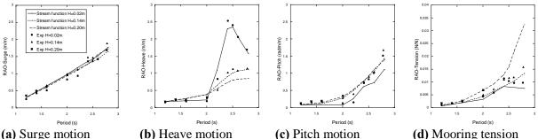
**Figure 3.** Comparison of RAOs of surge, heave and pitch motions, and mooring tensions between experiments and simulations in the intermediate water.
