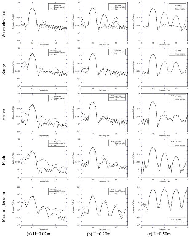
Figure 7. Comparison of PSD of normalized elevations, dynamic responses and mooring tensions, by linear and nonlinear wave theories for different wave heights.
