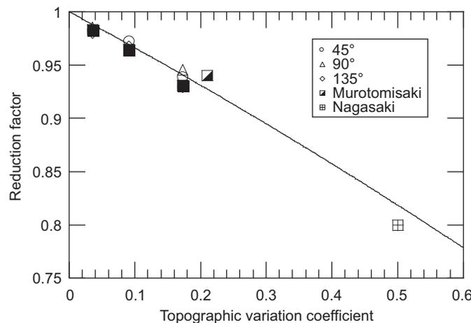
**Fig. 10.** Variation of reduction factors with topographic variation coefficients.
