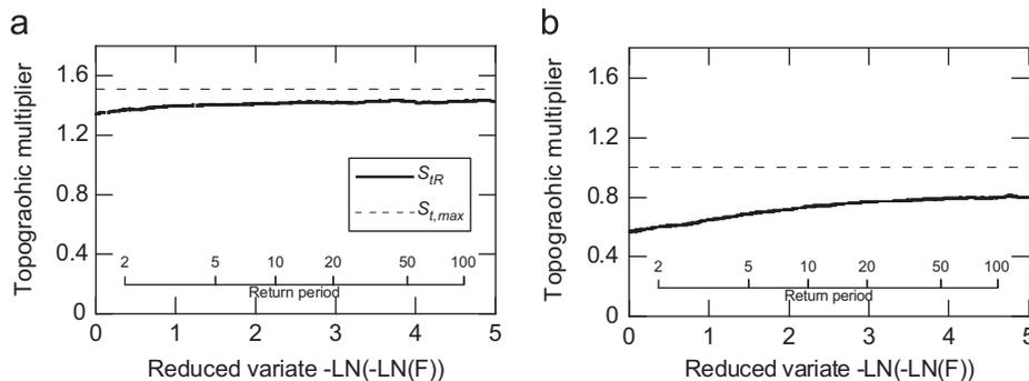
Fig. 6. Topographic multipliers with return period at (a) Murotomisak and (b) Nagasaki.
