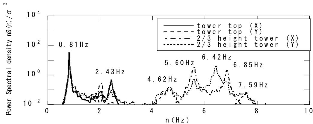
Fig. 4 Power spectral densities of the accelerations at the top and the height of 2/3 of the tower.
