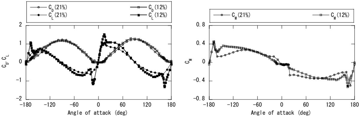
(a) Drag and Lift coefficients (b) Moment coefficient
