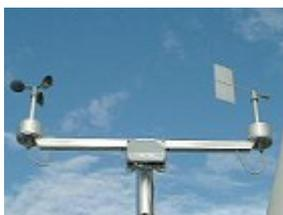
a) Anemometer and wind vane
