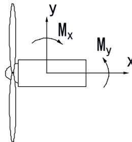
Fig. 7 Coordinate system for the tower bending moments
