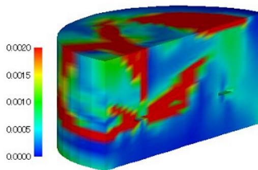
Fig. 18 Perspective view primary shear strain contour
