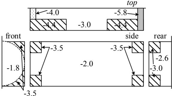
Fig.16 Schematic Distributions of Minimum Peak Pressure Coefficients for Panel Design Loads of Wind Turbine Nacelles ?
