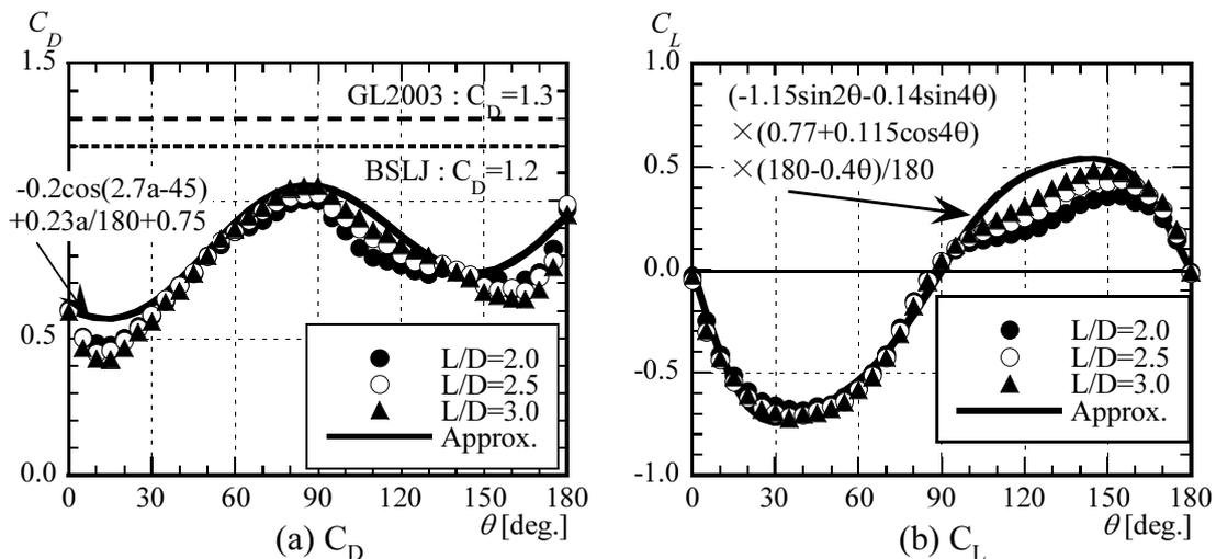
Fig.9 Effects of Hub Length on Nacelle Load( $A^{**}$  by eq.(4))
