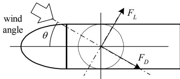
Fig.4 Definitions of Force and Wind Angle
