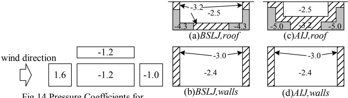
Fig.14 Pressure Coefficients for Nacelles in GL2003
