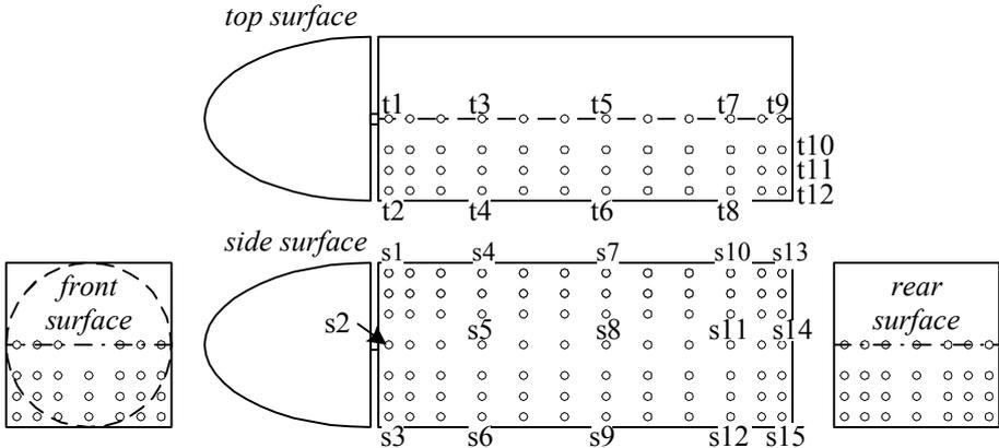
Fig.6 Pressure Measurement Points
