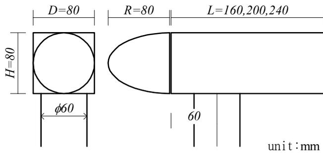
Fig.2 Experimental Model of Nacelle
