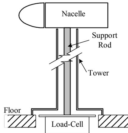
Fig.3 Setup of Model in Wind Force Measurements
