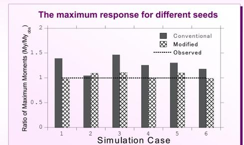
The results indicate that predicted maximum bending moments at the tower base show good agreements with measurements and correlation coefficients between observed and simulated moments increase from 0.143 to 0.603, when measured wind speed is used.
