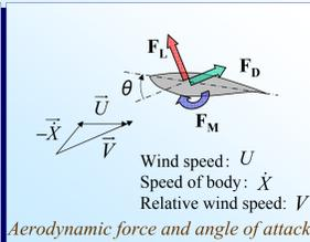
Aerodynamic force and angle of attack
