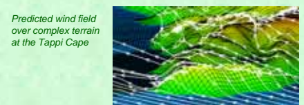
Predicted wind field over complex terrain at the Tappi Cape
