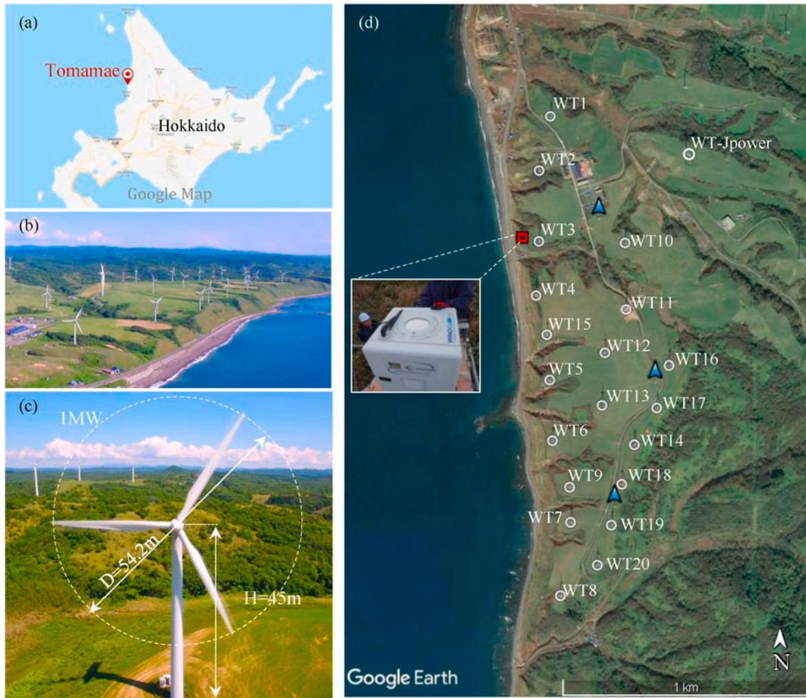
Fig. 3. Test site in the Tomamae wind farm: (a) location of Tomamae; (b) aerial picture of wind farm; (c) wind turbine and its dimensions; (d) layout of the wind farm and measurement where the white open circles denote the location of each wind turbine, the red square and the blue triangles indicate the position of LiDAR and Met-masts (No.1, No.2 and No.3 from north to south) respectively.
