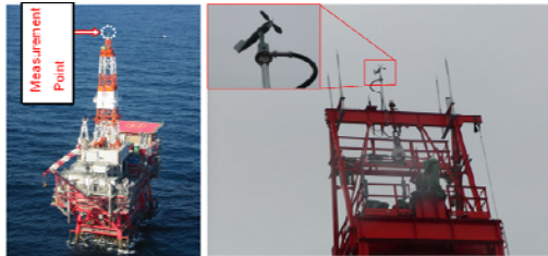
(a) A drilling derrick (b) Propeller-vane anemometer
