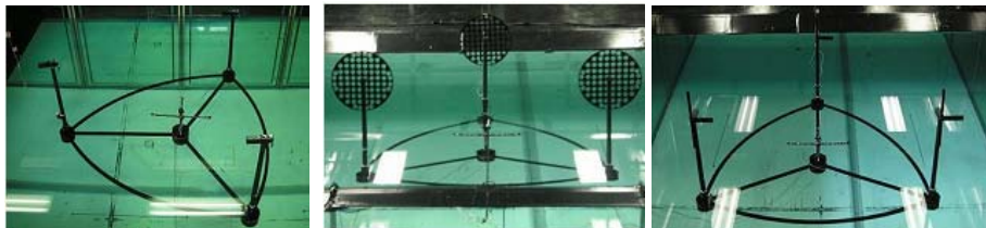
Figure 5. Experimental models (model with the rotors were modeled by the concentrated mass at the nacelles, in operating condition, in survival condition)
