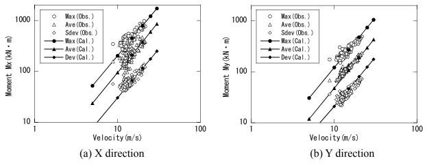
Fig. 10 Variation of tower bending moments with mean wind speeds in X and Y direction
