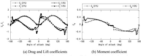
Fig. 8 Variation of aerodynamic coefficients with the angle of attack
