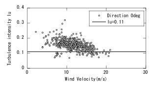
Fig. 3 Variation of turbulence intensities with mean wind speeds
