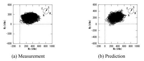
Fig. 9 Comparison of observed and predicted tower bending moments plotted in X-Y plane
