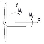
Fig. 7 Coordinate system for the tower bending moments
