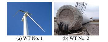
Fig. 5 Damaged turbines at Nanamata
