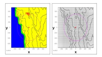
Fig. 13 Elevation contour, surface roughness and computational grid around Miyako branch office of Okinawa Electric Power Company
