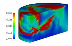
Fig. 18 Perspective view primary shear strain contour
