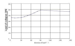
Fig. 21 Buckling Strength Against Direction of Load
