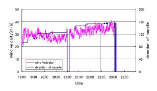
Fig. 8 Time series of yaw direction and the wind speed of turbine No. 5 at Karimata on September 10, 2003
