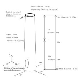
Fig. 19 The notation and the dimension of the tower model
