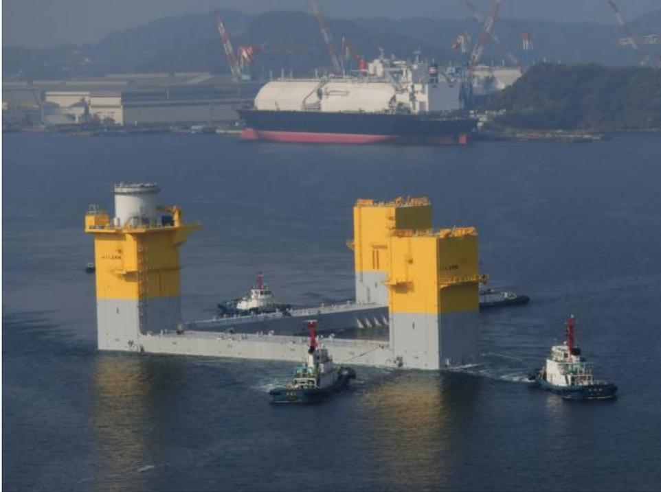
Towing of a three-column semi-sub, for the first 7MW wind turbine, from Nagasaki port to Onahama port will commence from November 1 and be completed on November 10.
